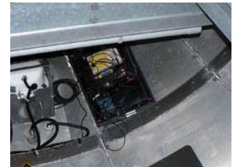
Remote microphone installed at the nacelle's bottom (above) and connected to automated bat detector inside the nacelle (below). © L. Bach
