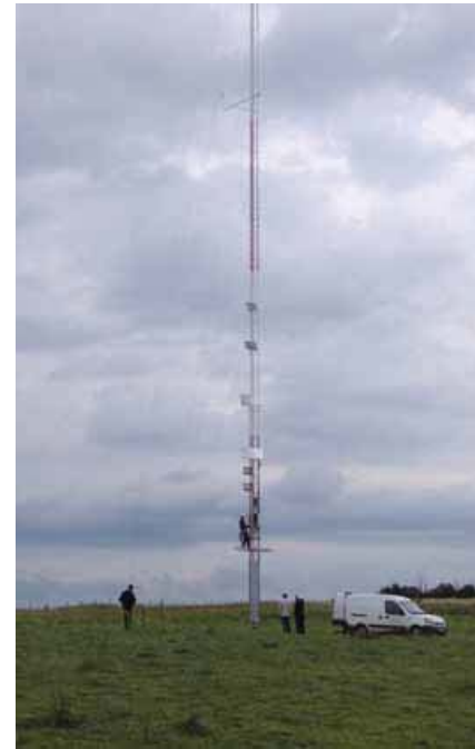
Meteorology mast with automated bat detectors installed for recording of bat activity at the height of the collision risk zone, France. © J. Sudraud
